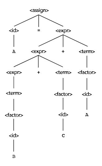
• The parse tree shows the left addition operator lower than the right addition operator. This is the correct order if addition is meant to be left associative.
