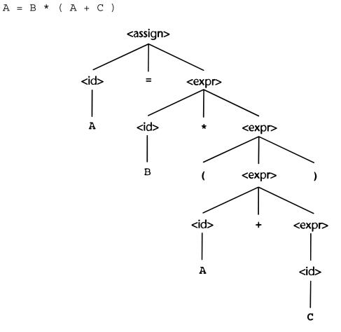
• Every internal node of a parse tree is labeled with a nonterminal symbol; every leaf is labeled with a terminal symbol.
